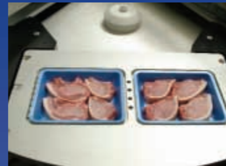
Quick change rotary tray carousel showing 2 up configuration.
