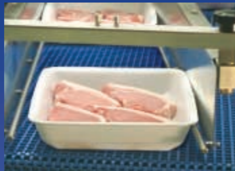
Optional diverger for automatic loading of trays into a multi-configuration sealing carousel.
